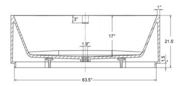
Note: ALL MEASUREMENTS ARE IN INCHES & HAVE TOLERANCE OF +/- 1/4"
