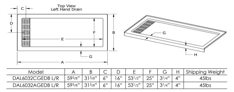
Note: ALL MEASUREMENTS ARE IN INCHES & HAVE TOLERANCE OF +/- 1/4"
