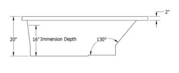
Note: ALL MEASUREMENTS ARE IN INCHES & HAVE TOLERANCE OF +/- 1/4"
