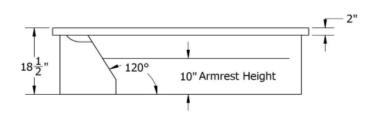
Note: ALL MEASUREMENTS ARE IN INCHES & HAVE TOLERANCE OF +/- 1/4"
