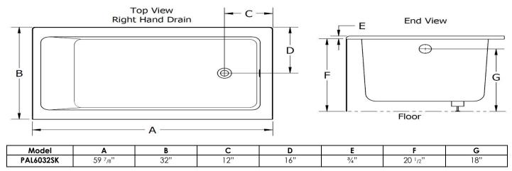
Note: ALL MEASUREMENTS ARE IN INCHES & HAVE TOLERANCE OF +/- 1/4"
