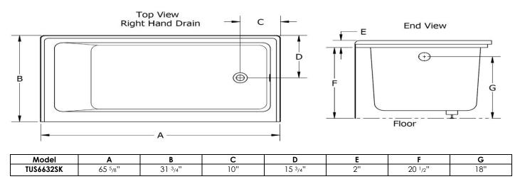
Note: ALL MEASUREMENTS ARE IN INCHES & HAVE TOLERANCE OF +/- 1/4"
