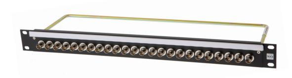
**FEATURES** - Using suitably rated BNC connectors these panels can be used up to 24GHz. The BNC connectors are isolated from the front panel and can have a density of up to 24 channels on a single row. With a redesigned aluminium extrusion, the designation strip is now clipped on to allow greater visibility and space for text.
