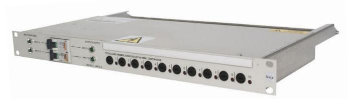
**OVERVIEW** - This unit safeguards equipment from primary mains supply failure with fast automatic changeover time. 12 individually fused IEC outputs are housed in a sturdy 19" 1RU rack mounted enclosure, 195mm behind panel depth (300mm including lacing bar).
