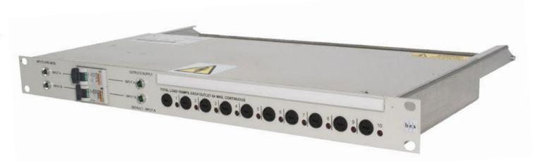
**OVERVIEW**—An integral EMC filter prevents radio frequency interference from reaching sensitive broadcast equipment. Protection against fast acting surges is also delivered to eliminate any possible effects from atmospheric disturbances or inductive switching elsewhere on the power network. Likewise, the filter will prevent any produced RFI, whether in switch mode power supplies or from microprocessors, from finding its way back onto the power supply and affecting other equipment.
