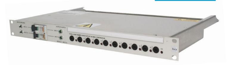
**FEATURES** - This mains distribution unit is housed in a 19" rack mounted chassis. 12 outputs are individually fused with power present LED's on the front panel. The unit features a loop 32 Amp Neutrik PowerCon inlet and two pole isolator mounted on the front panel. The front panel is made from extruded aluminium, finished in black with a wide clip-on designation strip for clear marking.
