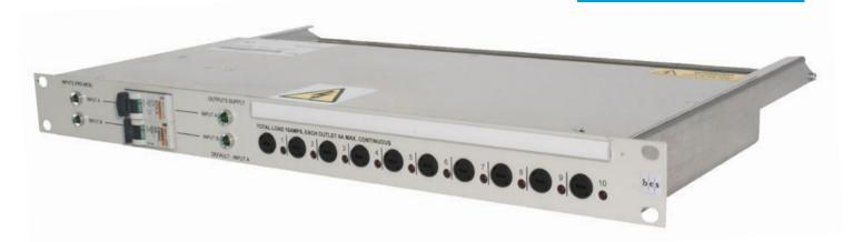
**FEATURES** - This mains distribution unit is housed in a 19" rack mounted chassis. 12 outputs are individually fused with power present on the front panel. The unit features a loop 32 Amp Neutrik PowerCon inlet and two pole isolator mounted on the front panel. The front panel is made from extruded aluminium, finished in black with a wide clip-on designation strip for clear marking.
