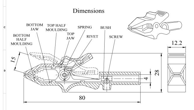
MATERIALS Noryl SE1 604 TOP HALF MOULDING TOP JAW B.M.S., Nickel plated Norvl SE1 604 BOTTOM HALF MOULDING BOTTOM JAW B.M.S., Nickel plated SPRING Spring Steel RIVET Brass BUSH Brass
