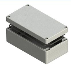
High Impact and Ingress Protection: Not only do they retain an impact rating of up to 7 joules, but all IP testing was carried out after impact testing, verifying that the seal is maintained when the enclosure is treated roughly. Most enclosures on the market perform IP testing before impact testing.
