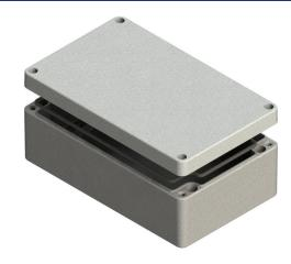
High Impact and Ingress Protection: Not only do they retain an impact rating of up to 7 joules, but all IP testing was carried out after impact testing, verifying that the seal is maintained when the enclosure is treated roughly. Most enclosures on the market perform IP testing before impact testing.
