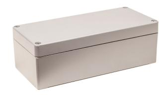
High Impact and Ingress Protection: Not only do they retain an impact rating of up to 7 joules, but all IP testing was carried out after impact testing, verifying that the seal is maintained when the enclosure is treated roughly. Most enclosures on the market perform IP testing before impact testing.
