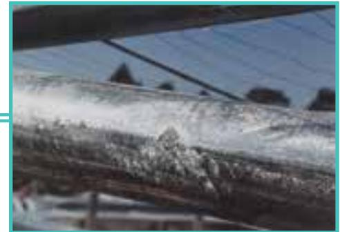
FIGURE 25: TOUCH MARKS (REJECTABLE)
