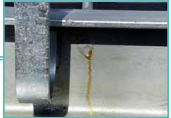
FIGURE 33: WEEPING WELD (ACCEPTABLE)
