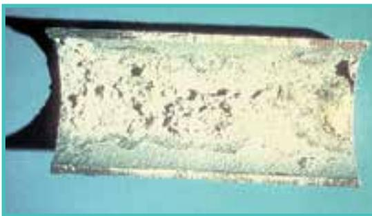
FIGURE 22: FLUX INCLUSIONS FROM INTERIOR OF PIPE (REJECTABLE)
