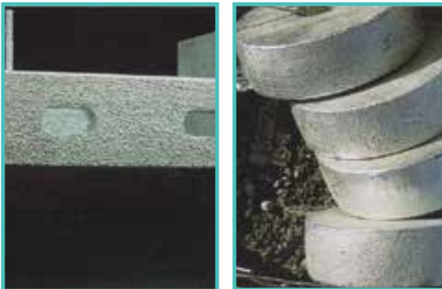
FIGURE 26: ROUGH SURFACE CONDITION/ STEEL SURFACE CONDITION (ACCEPTABLE)
