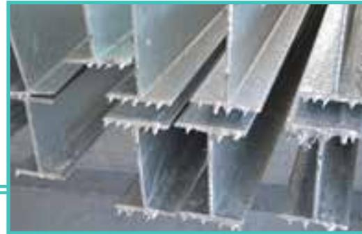
FIGURE 18: DRAINAGE SPIKES (ACCEPTABLE AFTER REMOVAL OR FILING)
