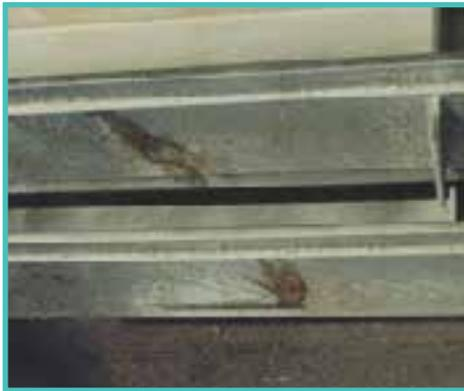
FIGURE 34: WELDING BLOWOUT (REJECTABLE)
