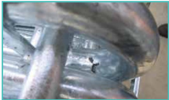
FIGURE 12: BARE SPOTS (REJECTABLE)
