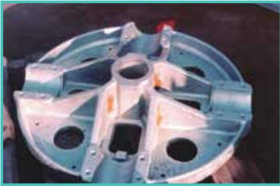
FIGURE 29: SAND EMBEDDED IN CASTING (REJECTABLE)
