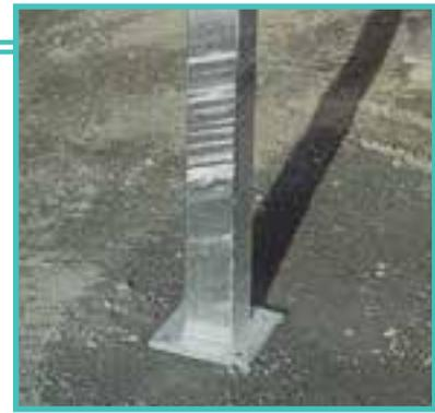
FIGURE 23: OXIDE LINES (ACCEPTABLE)
