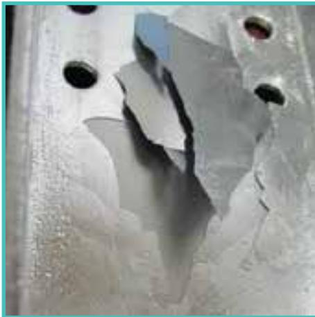
FIGURE 21: FLAKING (REJECTABLE)
