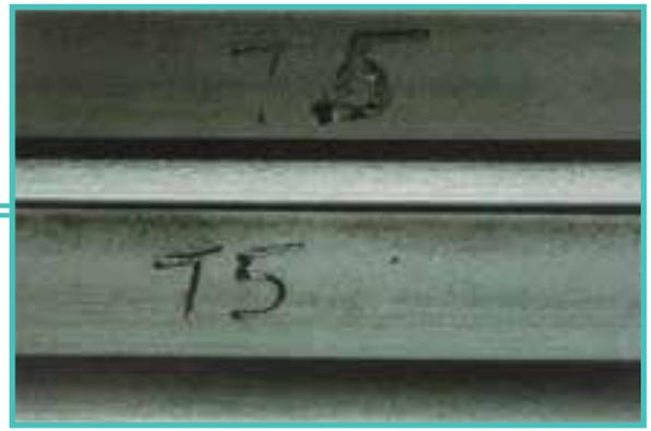
FIGURE 32: SURFACE CONTAMINANT (REJECTABLE)
