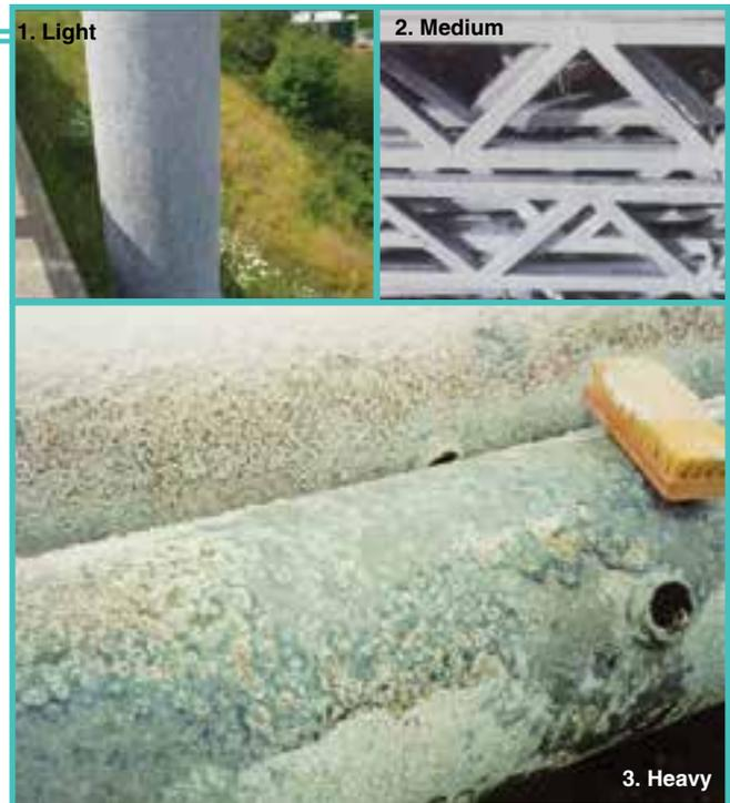
FIGURE 36: WET STORAGE STAIN (LIGHT (1) OR MEDIUM (2) IS ACCEPTABLE, HEAVY (3) IS REJECTABLE)
