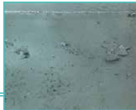
FIGURE 38: ZINC SPLATTER (ACCEPTABLE)
