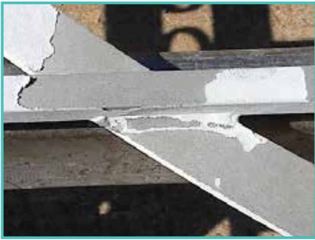
FIGURE 13: BLASTING DAMAGE (REJECTABLE)
