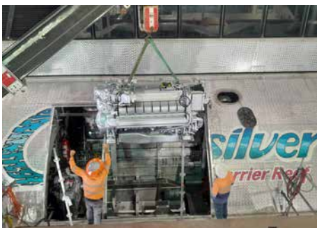
Quicksilver V repower: With the old engines removed via an opening cut into the aluminum hulls, the new engines are craned into position.
