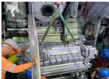
Quicksilver V repower: With the old engines removed via an opening cut into the aluminum hulls, the new engines are craned into position.
