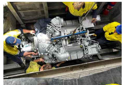
Poseidon dive & snorkel catamaran new generation engines being installed.
