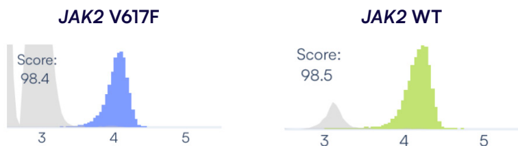
Figure 1. Representative fluorescence intensity histogram for the Countable JAK2 V617F assay, showing clear separation between target signal (JAK2 V617F: blue; JAK2 WT: green) and background (grey). The Intensity Distribution (ID) score for each target appears in the upper-left corner, demonstrating strong signal-to-noise performance.
