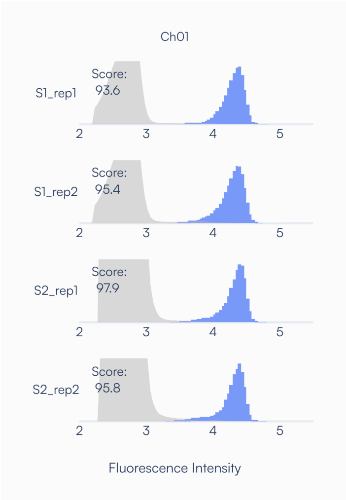
Figure 3. Fluorescence intensity histograms for WPRE assay from samples and technical replicates in the Countable PCR data summary. Each trace displays a distinct amplification profile with automatically generated ID Scores (93—98) confirming strong signal discrimination. Every Countable PCR run produces this standardized report with full plots and QC metrics stored in a 21 CFR Part 11—compliant format, supporting GMP-ready traceability.
