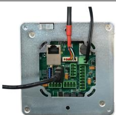
Now wire the relay(s) to your door circuit. For this you need a power cable, which transmits the impulse to the door / gate etc. This cable is usually supplied with the door and it is a low-voltage cable.
