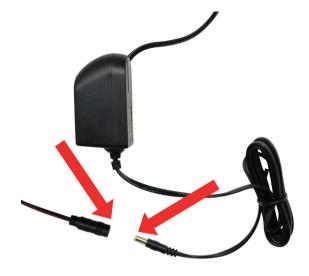
Finally, to get your system up and running, connect the controller to the power supply.
