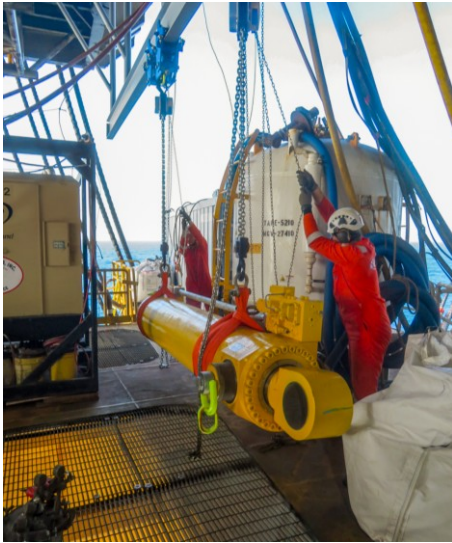
Lifting cylinder with rigging gear
