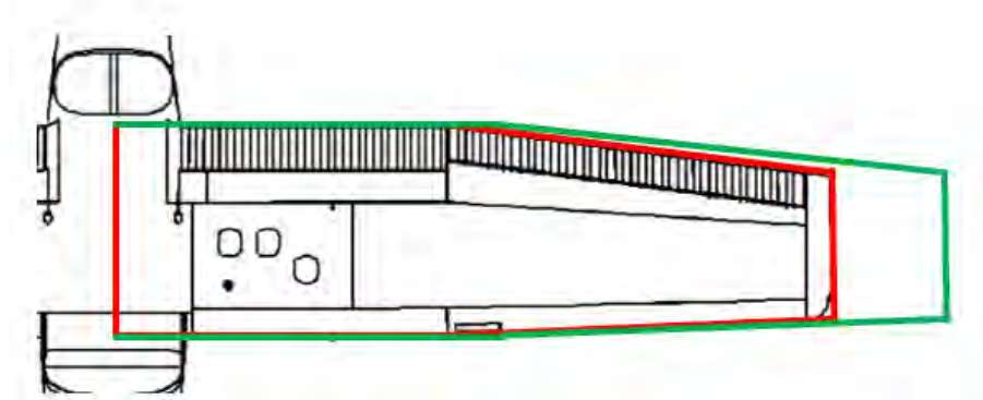
Figure 7.1: Increase of 15% in wingspan. New wing planform shown in green, compared to the original in red.
