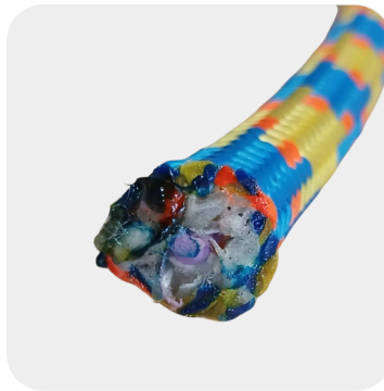
✘ Rope end not well sealed
