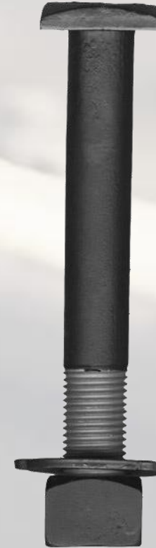
SWITCH & CROSSING 'V' GRADE BOLT (thin head) Complete with Renlok nut and through hardened washer Part No. 57/023499 1" X 7 3/4" 57/023500 1" X 8"
