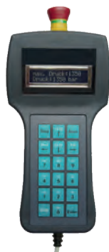
Pressure ITH High Pressure Pump with APC control
