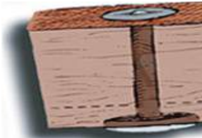
How the rivet was used to hold the timbers in place.
