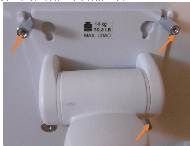
Figure 24: PC with 3 hex-standoffs and the knurled nut
