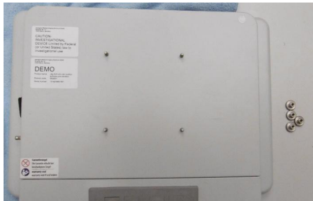
Figure 23: Take off the knurled nuts from the PC
