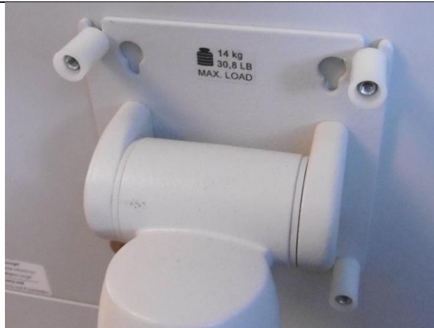
Figure 27: 3 isolation pieces over the 3 hex standoffs
