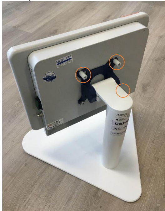
Figure 41: 3 isolation pieces over the 3 hex standoffs
