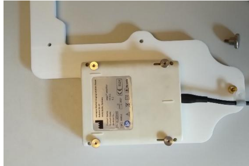
Figure 21: USB cable connected to the amplifier without the drag protection tightened
