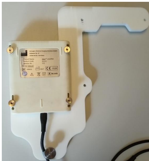
Figure 22: USB cable now tighten with the knurled nut to complete the drag protection
