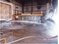
The SuperVault MH is the first Multi-Hazard Rated Insulated and Protected Above Ground Petrol Storage Tank available in the world and it is the first tank to pass the stringent safety requirements of Uniform Fire Code Standard A-II-F-1 (formerly known as 79–7) and Southwest Research Institute Standard 95–03 and 93–01.The multi-hazard rating allows the Supervault MH to be re-certified for use after exposure to a fire, puncture or impact.
