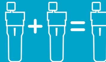
The UD+ combines two filtration steps (DD+ and PD+) into one, a unique technology to meet the quality requirements of diverse applications and offer superior energy savings. The UD+ filter provides the same air purity as a DD+PD+ filter train with a lower pressure drop.
