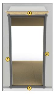
The sub-floor area must be at least: 6" deep for 4-9/16" frames 8" deep for 6-5/8" frames.
