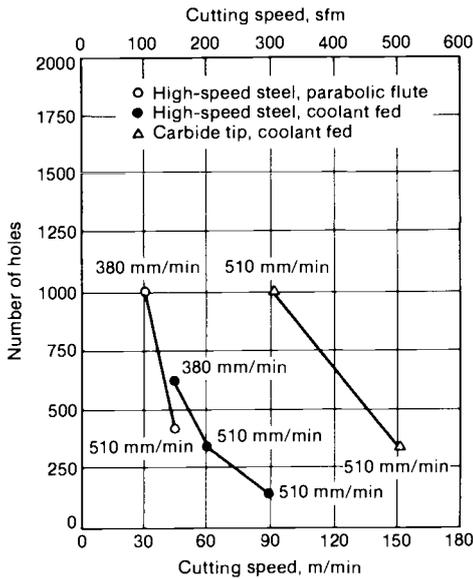
**Fig. 21** Drill life at various penetration rates for several types of drills when drilling permanent mold 390 aluminum alloy. Source: Ref 2
