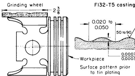
Machine . . . . . Cylindrical grinder, 152 × 457 mm (6 × 18 in.), with automatic infeed electric-cycle control and semiautomatic profile dresser
