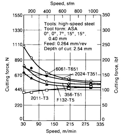
**Fig. 5** The effect of speed on cutting force for five aluminum alloys
