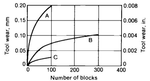
**Fig. 29** Tool wear curves for the single-tooth milling of alloy 390 engine blocks (wet) at 0.30 mm/rev (0.012 in./rev), A, carbide, 150 m/min (492 sfm); B, diamond, 1500 m/min (4920 sfm); C, diamond, 150 m/min (492 sfm). Source: Ref 2
