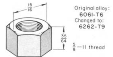
**Fig. 4** Hexagonal nut for which a change from alloy 6061-T6 to 6262-T9 resulted in a savings of material and less burring of the tapped thread. Dimensions given in inches
