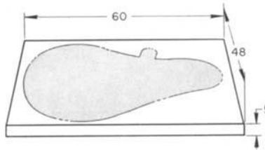
**Fig. 32** Shape that was contour band sawed from aluminum plate. Dimensions given in inches
