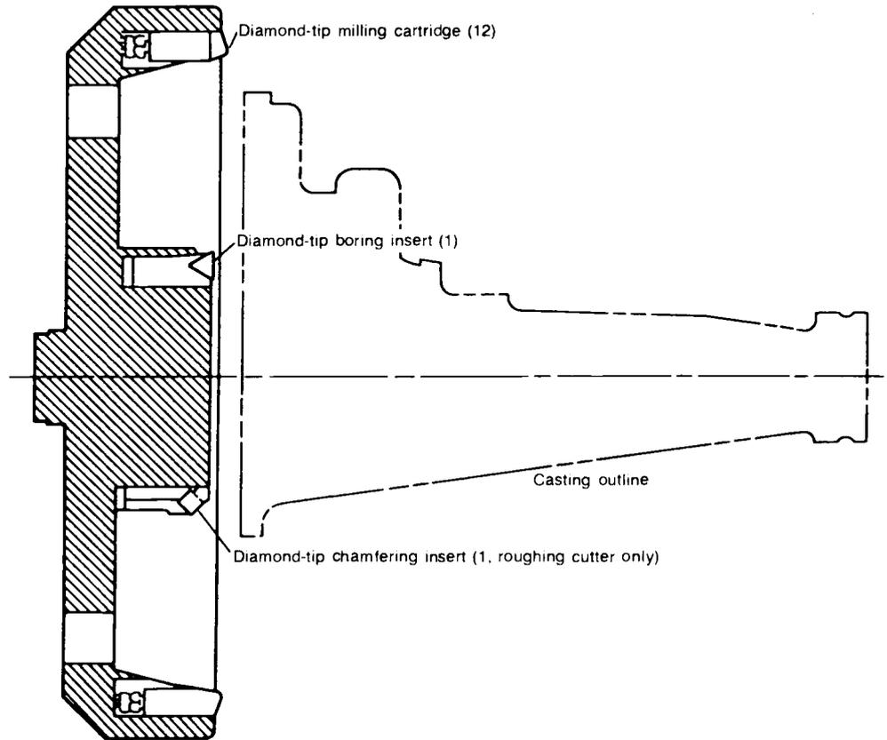
**Fig. 31** Schematic of a combination boring-milling cutter with diamond-tip cutters machining a 380 aluminum alloy transmission extension housing at 3840 m/min (12 600 sfm)
