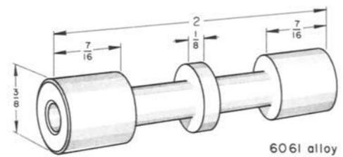
**Fig. 35** Part from which 0.005 mm (0.0002 in.) of metal was removed by lapping to smooth the surface to 0.025 μm (1 μin.). Dimensions given in inches
