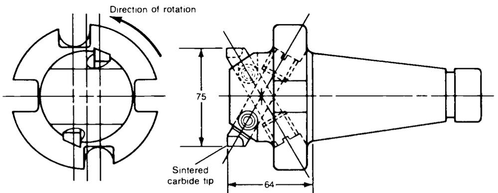
**Fig. 24** Special two-cut tooth end mill with sintered carbide cutters. Dimensions given in millimeters. Source: Ref 4
