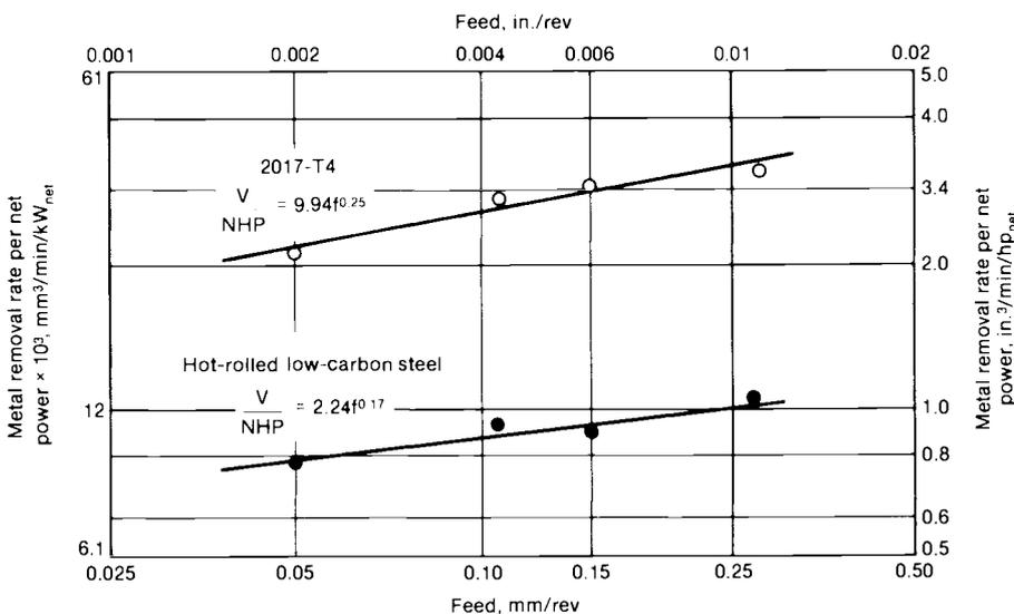
**Fig. 3** The effect of feed on metal removal rate per net power for low-carbon steel and aluminum alloy 2017-T4 with comparable mechanical properties. V/NHP, volume per net horsepower
