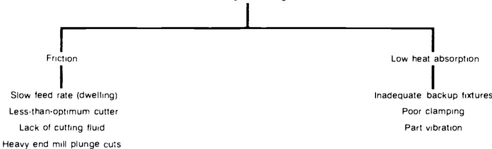
**Fig. 13** Causes of overheating during machining process attributable to friction and low heat absorption problems
