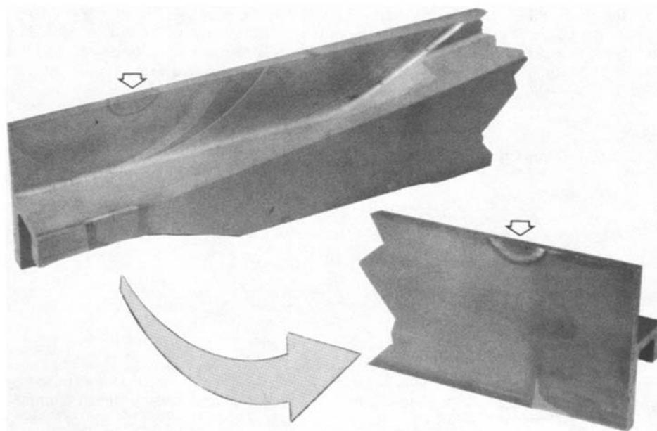
**Fig. 6** Typical spar mill defect at a section change. Courtesy of McDonnell Douglas Canada, Ltd.
