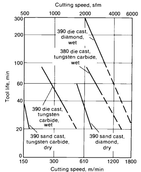
**Fig. 14** Tool life curves for the dry turning of sand cast alloy 390 using carbide and diamond, the wet turning of die cast alloy 390 using carbide and diamond, and the wet turning of die cast alloy 380 using carbide. Source: Ref 2
