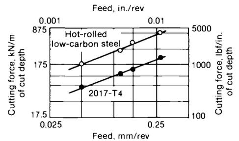
**Fig. 2** The effect of feed on cutting force for low-carbon steel and aluminum alloy 2017-T4 with comparable mechanical properties
