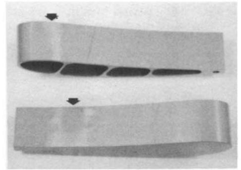
**Fig. 12** Two views of a milling defect on an unsupported vertical flange in a 7075-T651 aluminum plate. Courtesy of McDonnell Douglas Canada, Ltd.
