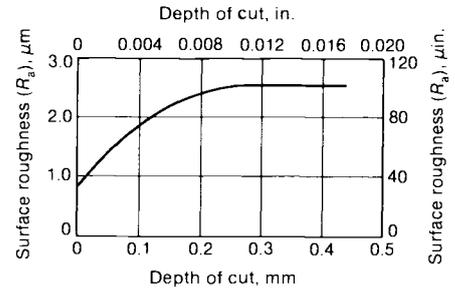
**Fig. 36** Relationship between surface finish and depth of cut for the chemical milling of 7075 aluminum sheet. Source: Ref 5
