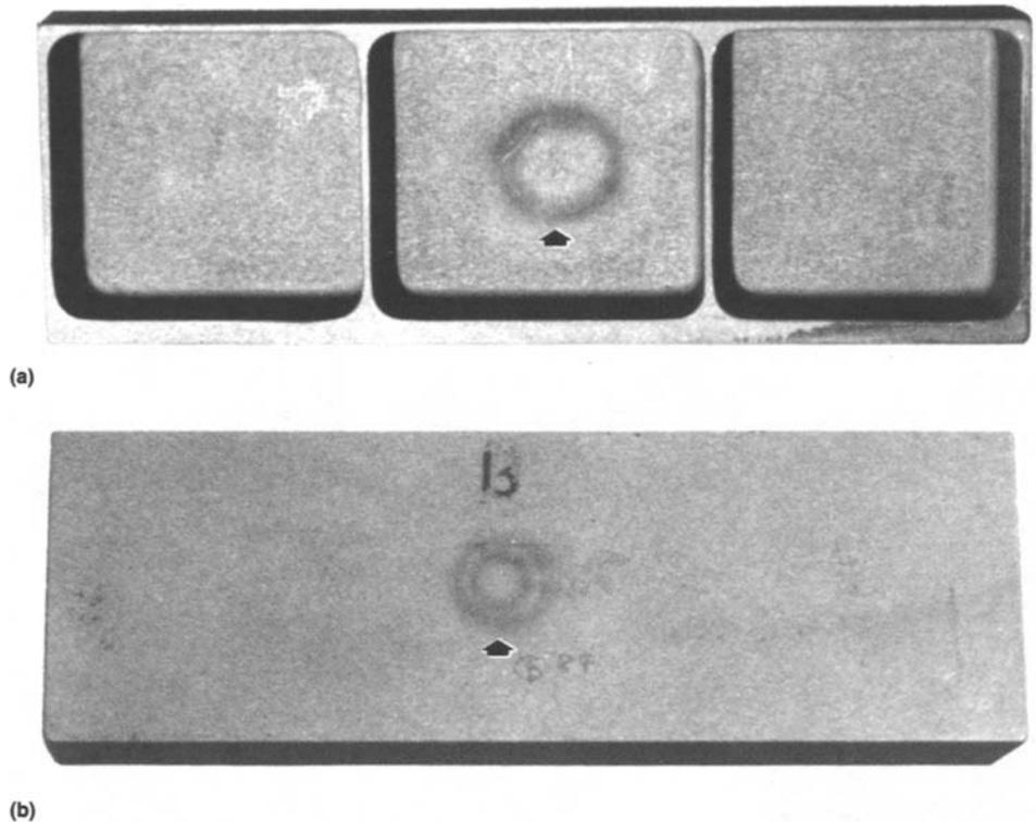
**Fig. 7** Typical end mill defect associated with vertical plunge cut pocketing operations. (a) Frant view. (b) Back view. Courtesy of McDonnell Douglas Canada, Ltd.
