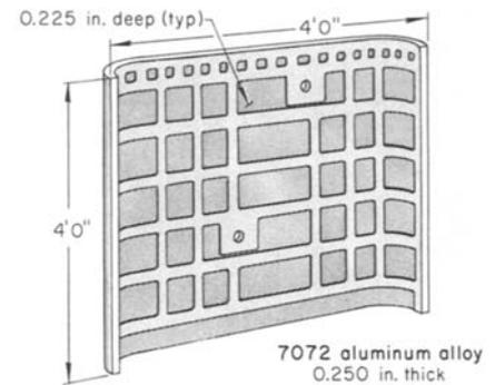
**Fig. 37** Preformed aircraft skin section chemically contoured to reduce weight. Dimensions given in inches
