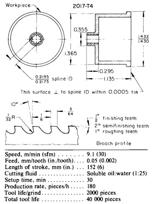
**Fig. 16** Clutch housing and details of broach used for producing the internal splines. Dimensions in figure given in inches
