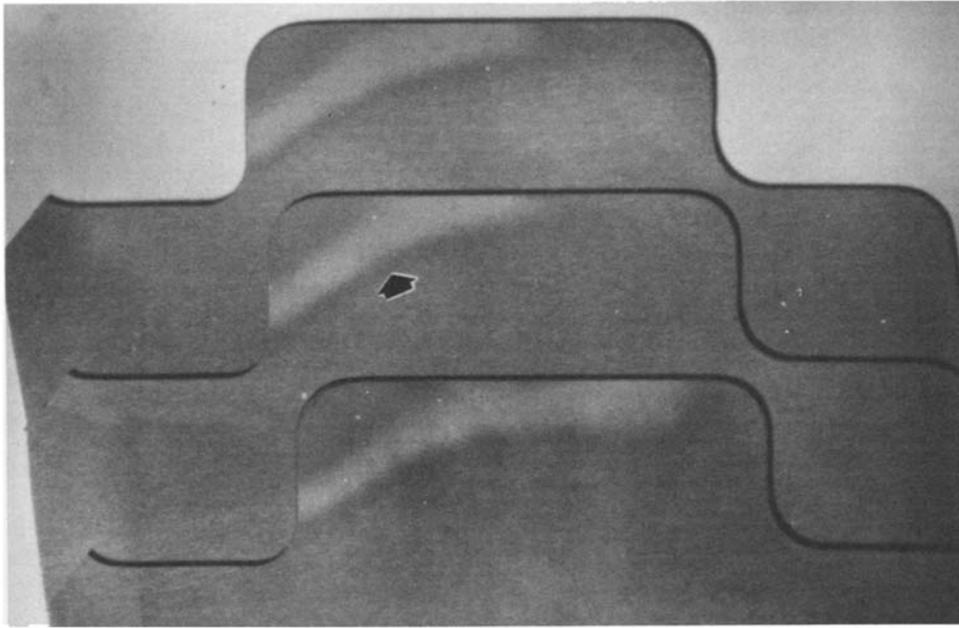
**Fig. 11** Occurrence of soft spots in the same location on each of three 7075-T651 aluminum plate components. Of the 19 parts produced, 13 had a soft zone hardness of 68 to 87 HRB and conductivity of 36 to 39%. Unaffected regions of the plate had a hardness of 90 to 91 HRB and conductivity of 31 to 32%. Courtesy of McDonnell Douglas Canada, Ltd.
