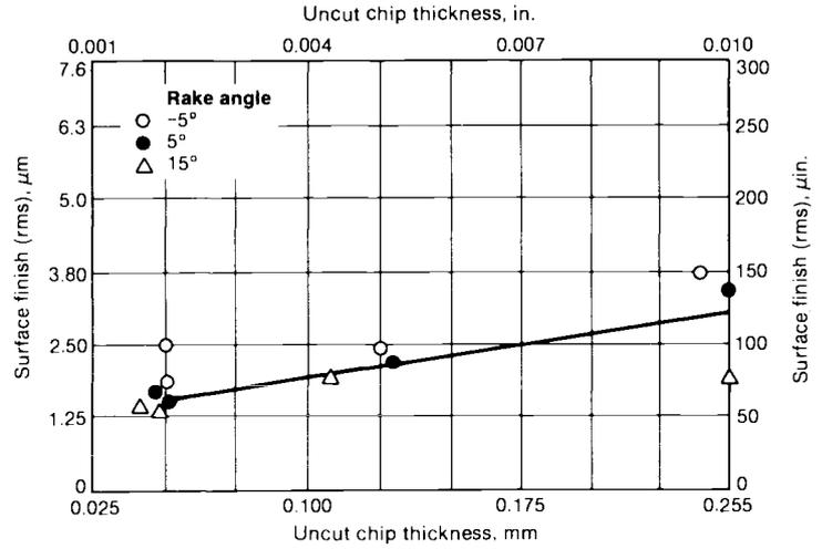
**Fig. 18** Surface finish at various depths of cut when broaching 390 aluminum alloy of 100 HB at 45 m/min (150 sfm) with a carbide tool. Although the rake angle varied, the shear angle of the tool was 0° in all three cases. Source: Ref 2
