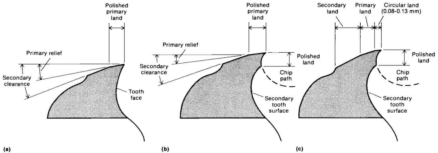
**Fig. 23** Three end mill geometries designed for the cutting of aluminum alloys. (a) Conventional milling. (b) Heavy metal removal. (c) Finishing operations. Source: Ref 1
