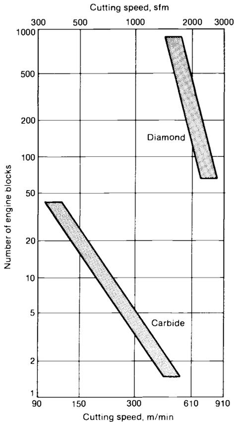
**Fig. 30** Tool life of carbide and diamond tools when milling alloy 390 engine blocks (dry). Source: Ref 2
