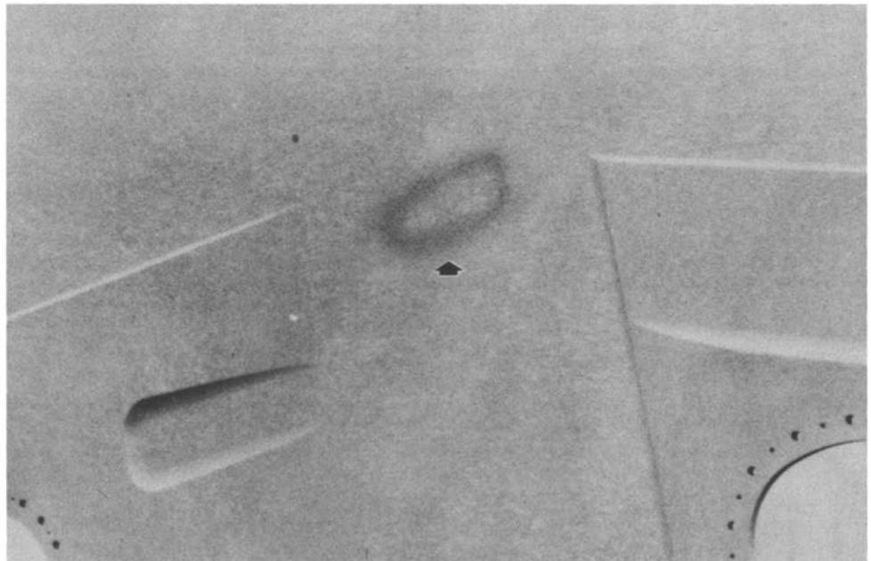
**Fig. 8** Milling defect associated with the NC machining of 7075-T7651 aluminum plate with a 75 mm (3 in.) diam milling cutter. Courtesy of McDonnell Douglas Canada, Ltd.
