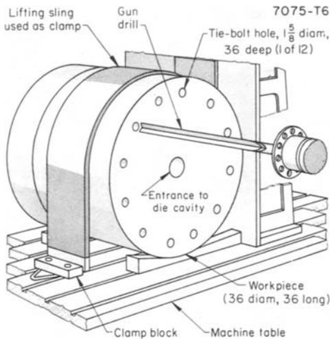
**Fig. 19** Setup for deep-hole drilling an explosive forming die in a boring mill. Dimensions given in inches
