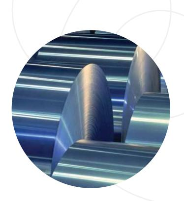
recoil it after each rolling pass, ready for the next, until the required thickness is obtained. Annealing may be required between passes depending on the final temper (hardness) required.
