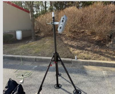
Example of permanent outdoor mounting with elevated radio and 30 downward degree tilt.
