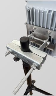
Radio mounted to tripod using mounting bracket.
