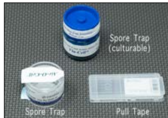
Figure 6. Air and surface sample collection devices
