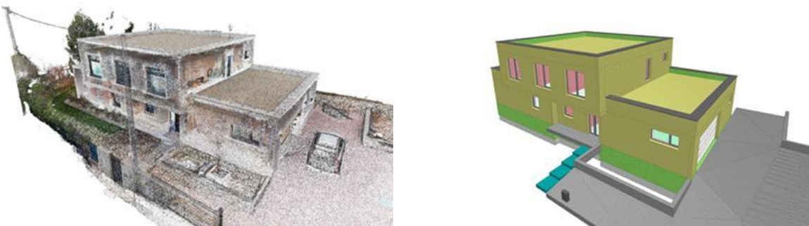
Fig. 5.14 Input georeferenced point cloud (left) and the resulting detailed BIM model (right), RD Zobor case study
