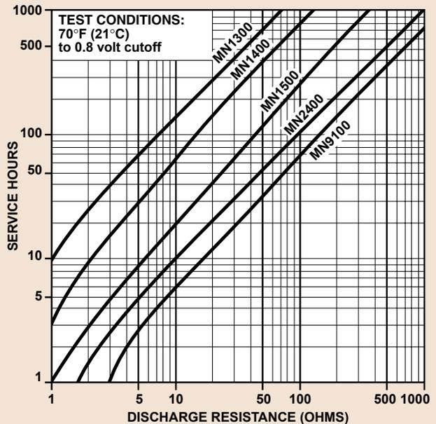
Typical discharge characteristics with constant resistance of DURACELL® alkaline cells.
