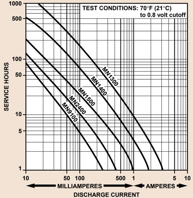
Typical discharge characteristics with constant current of DURACELL® alkaline cells.
