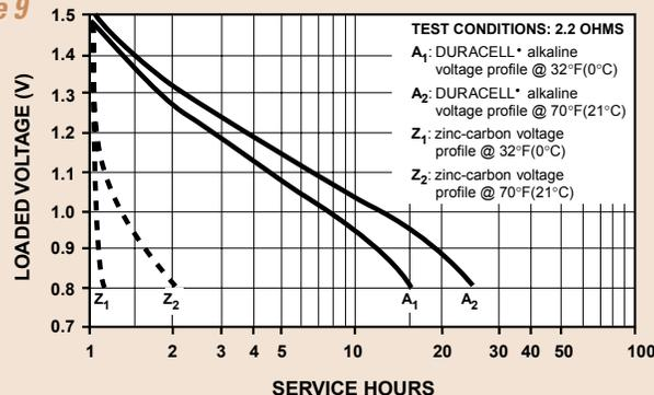
Comparison of the effects of temperature on a regular zinc-carbon "D" size cell versus a DURACELL® alkaline MN1300 ("D" size) cell.
