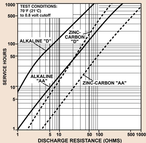
Comparison of the typical discharge characteristics of regular zinc-carbon "D" and "AA" size cells versus DURACELL® alkaline "D" (MN1300) and "AA" (MN1500) size cells.
