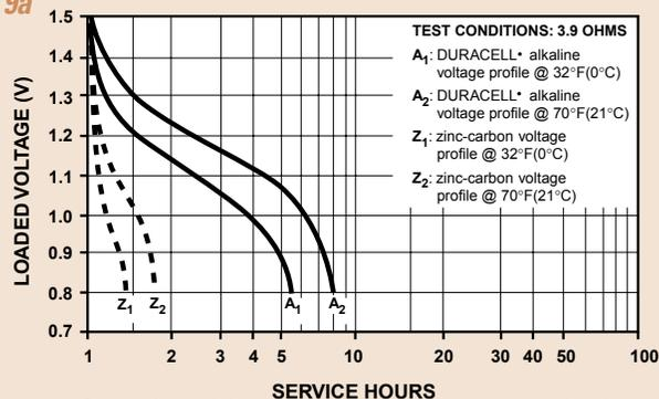
Comparison of the effects of temperature on a regular zinc-carbon "AA" size cell versus a DURACELL® alkaline MN1500 ("AA" size) cell.
