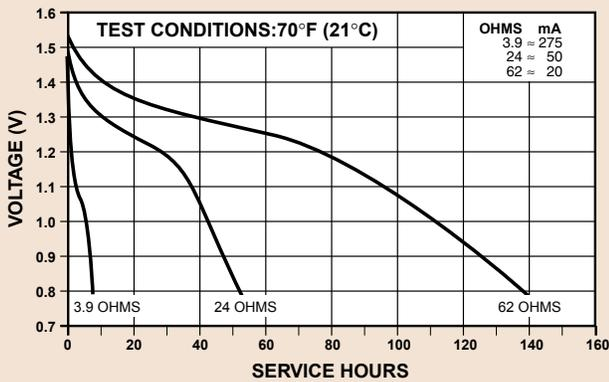
Typical discharge profile of the DURACELL® alkaline MN 1500 ("AA" size) cell.
