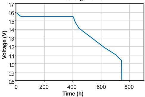
Constant Load: 6.8 k $\Omega$ Starting Drain: 229  $\mu$ A Temperature: 20°C
