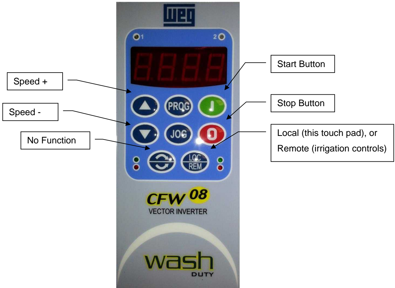
Figure 10: VFD Touchpad Detail
