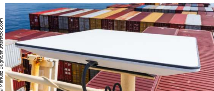
Example of OTM flat panel antenna mounted on board of big container ship.
