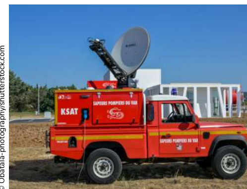
Example of an OTP terminal mounted on a trailer for firefighter operations in France.
