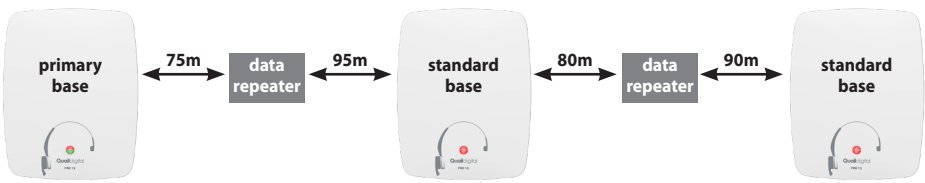
figure 8 - Adding data repeaters to base daisy chain
