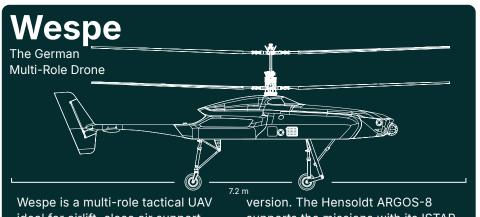
ideal for airlift, close air support and medical evacuation in land operations and naval scenarios. With its piston engine, the drone offers a range of 300 km and a total payload of 200 kg, which can be upgraded to 350 kg in the turbine
