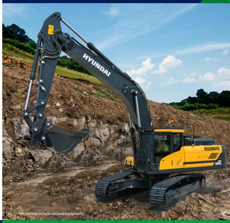
Gross Power 209 kW (280hp) at 2,200 rpm **Net Power** 205 kW (275hp) at 2,200 rpm
