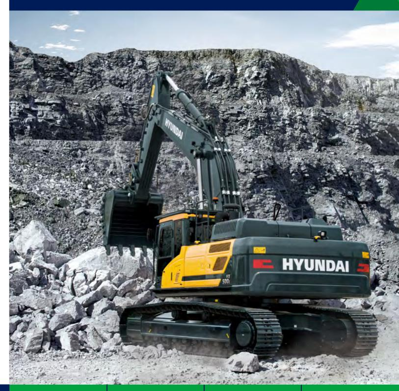
Gross Power 250 kW (335 HP) at 2100 rpm **Net Power** 246 kW (330 HP) at 2100 rpm Bucket Capacity 1.38 ~ 3.20 m<sup>3</sup> Operating Weight 49,900 kg
