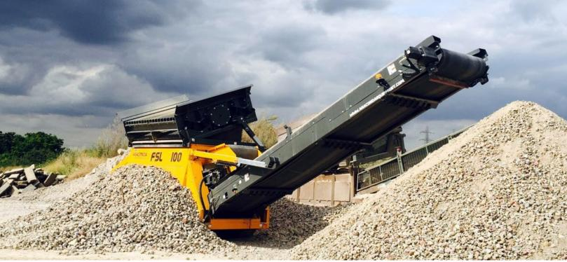
The Anaconda FSL Range of Mobile Tracked Scalping Screens are Heavy Duty Screens that have been developed specifically to suit the most difficult of applications.
