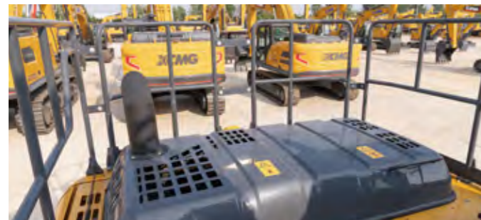
HANDRAILS AND GUARD RAILS
