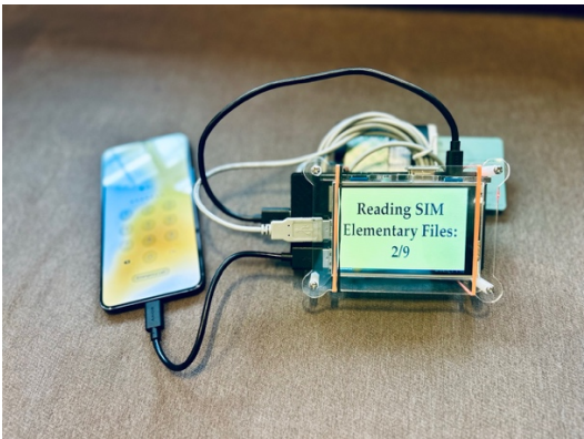
Figure 4Full miniaturized kit, Rasp3 SBC with display, battery, and SIM card programmer
