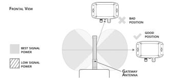
Keep the node and the gateway in line of sight as much as possible, as obstacles along the path of the signal could have a negative impact on the radio link.
