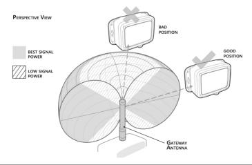
Avoid, if possible, to locate the gateway vertically above or under the node. If this cannot be avoided, it is best to keep the two antennas perpendicular to one another.
