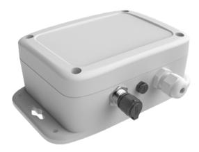
This communication device can read and digitize geotechnical sensors in static regime such as: strain gauges, temperature sensors, load cells, crack meters, humidity sensors, piezometers, anemometers, inclinometers, rain gauges and radar-based probes among others. These sensors can be purchased through Move Solutions™ or other channels.
