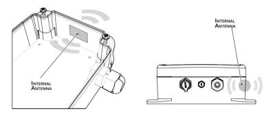
For optimal radio performance, the antenna should be oriented the same way as the gateway antenna, and the gateway should be on the side of the node.
