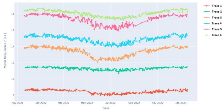
Fig 4: Modal frequencies during the first year of monitoring
