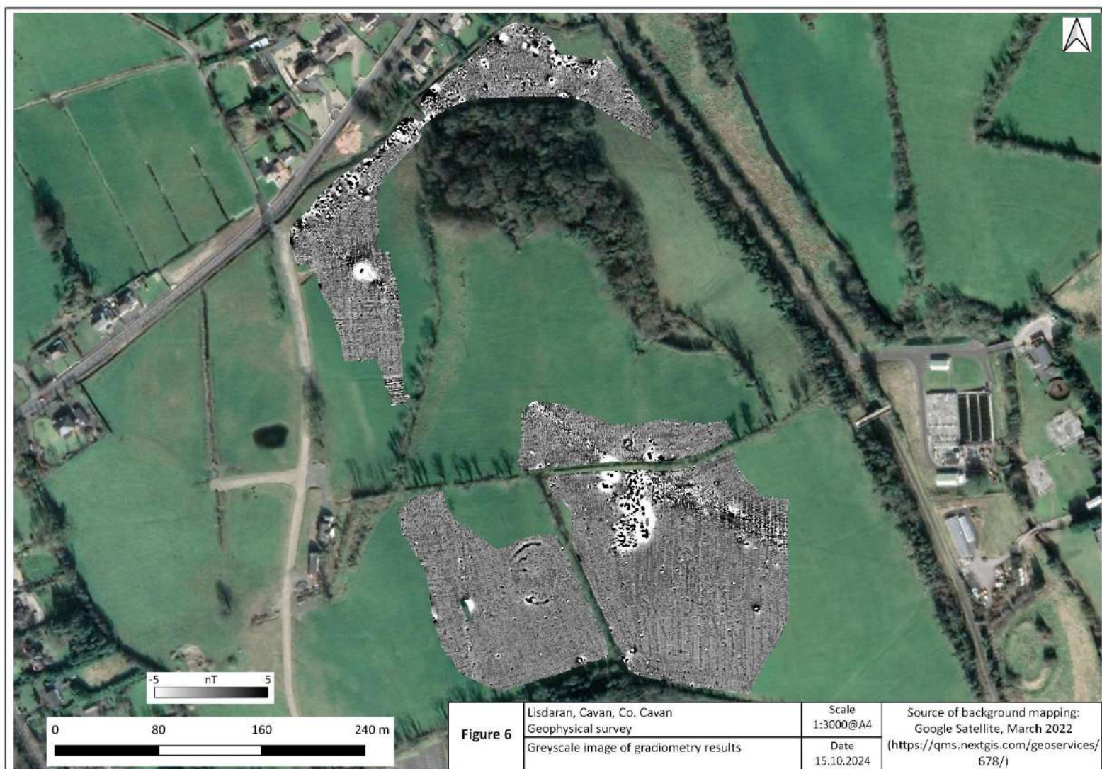
Figure 6. Greyscale image of gradiometry results.
