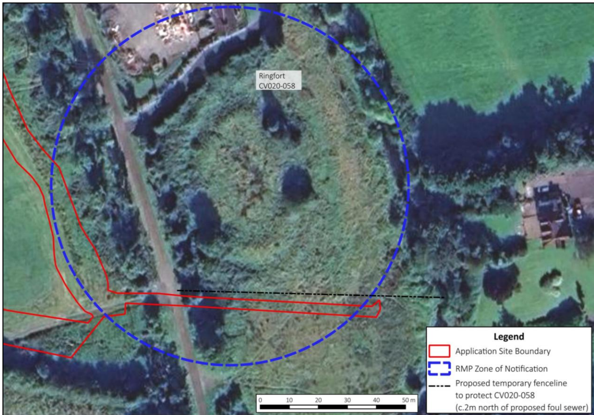
FIGURE 3: Proposed temporary fenceline to protect monument CV020-058 during construction
